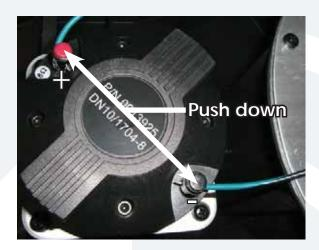
The positive (solid blue) and negative (blue and black) cables are still attached to the high frequency driver terminals. Remove the cables from their terminals simply by pushing down on the terminal and pulling out the cable.
